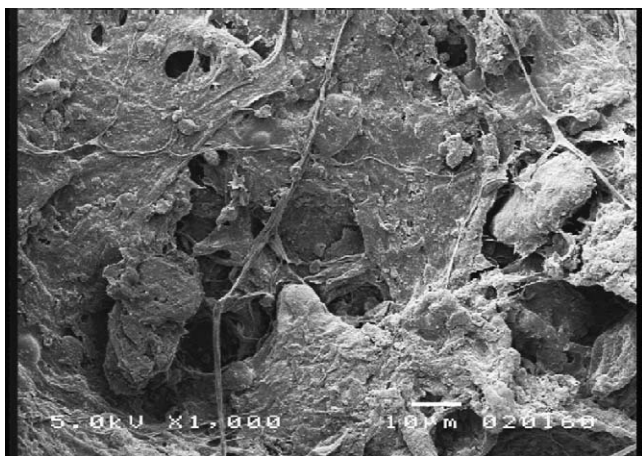
Fig. 3. SEM micrograph of the particles of waste acorn after Cr(VI) adsorption (pH 2.0, initial Cr(VI) concentration = 100 \text{ mg l}^{-1} , particle size = 0.5–1.0 mm, flow rate = 10 \text{ ml min}^{-1} ).
